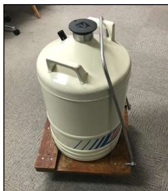
Figure 11: Left: Liquid nitrogen dewar and trolley. Right: Appropriate positioning of liquid nitrogen dewar with respect to the magnet.
