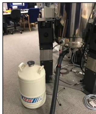
Figure 11: Left: Liquid nitrogen dewar and trolley. Right: Appropriate positioning of liquid nitrogen dewar with respect to the magnet.
