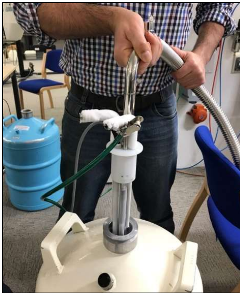
Figure 16: Inserting the N 2 exchanger into the LN 2 Dewar.
