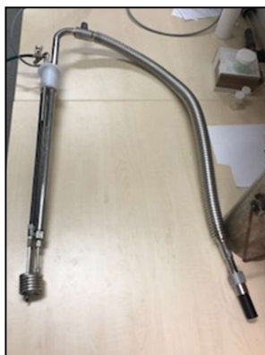
Figure 12: Nitrogen exchanger and transfer line for low temperature NMR.
