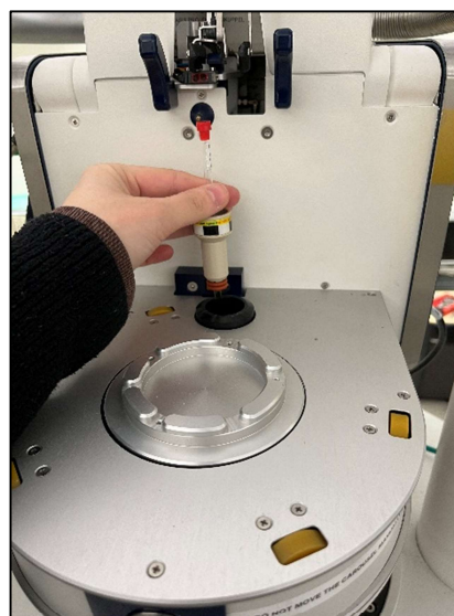
Figure 4: Manual sample insertion: Left: the BSMS panel and Right: sample insertion to the AVB500 magnet bore.
