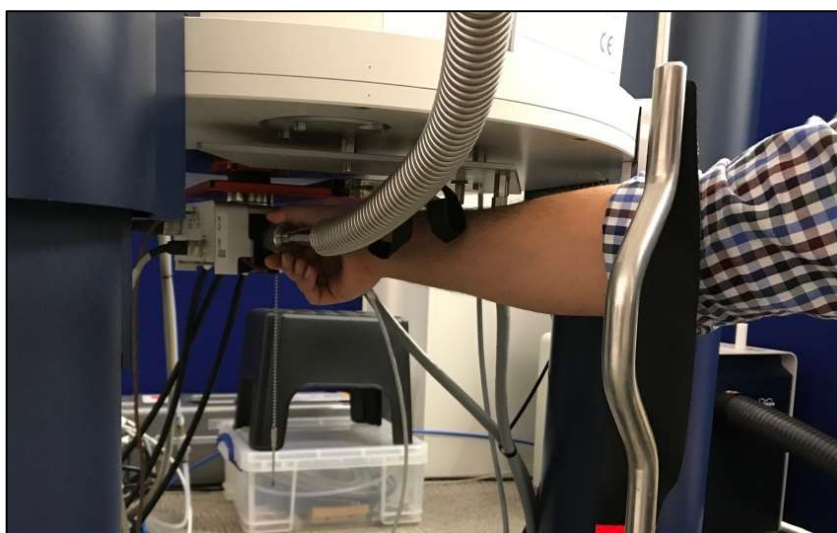
Figure 17: Insertion of the N 2 exchanger transfer line into the probe.
