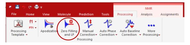
Zero filling increases the apparent acquired length of the FID, resulting in higher digital resolution and a "smoother" spectrum
