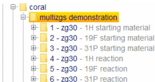
3. Having run the first reaction spectrum, open the first experiment run of the kinetic study (in this case, experiment 4) and use the command **multizgs** (answer the following questions).
