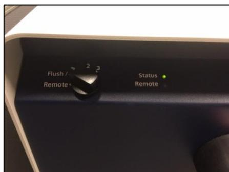
**Figure 5:** Turning off the chiller units on the AVB500 and AVX500- turn dial to **Flush**.
