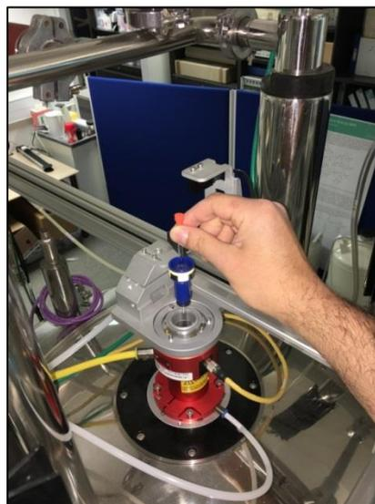
**Figure 4:** Manual sample insertion: *Left:* the BSMS panel and *Right:* sample insertion to magnet bore.
