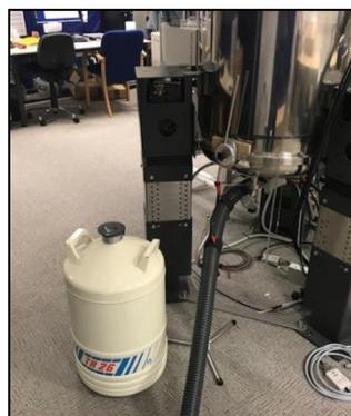
**Figure 10:** *Left:* Liquid nitrogen dewar and trolley. *Right:* Appropriate positioning of liquid nitrogen dewar with respect to the magnet.
