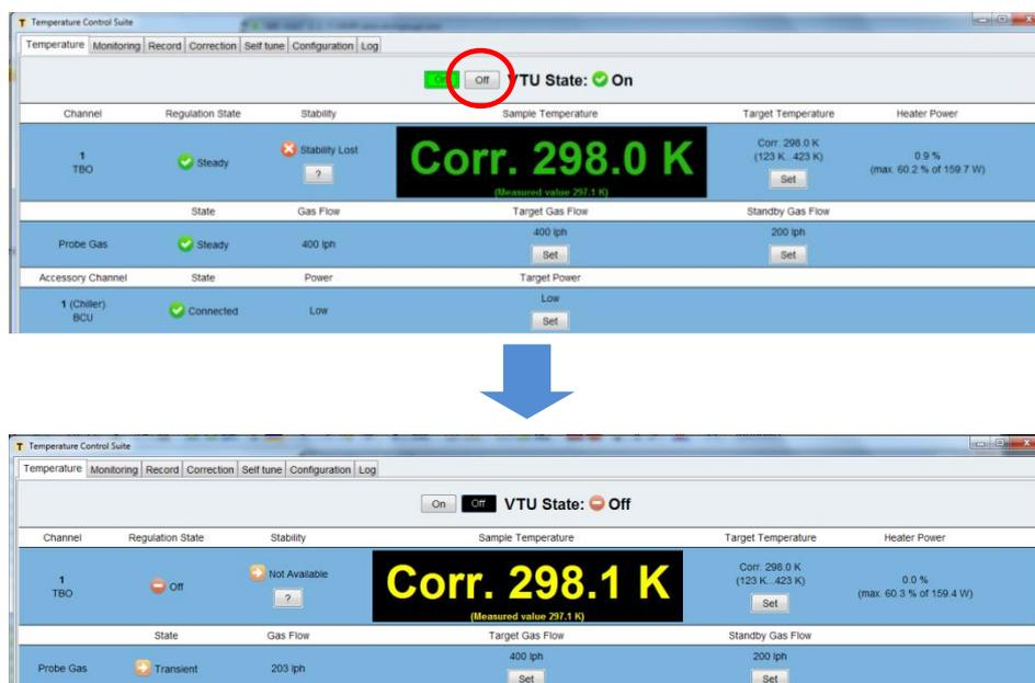
**Figure 13:** Turning off the VTU.
