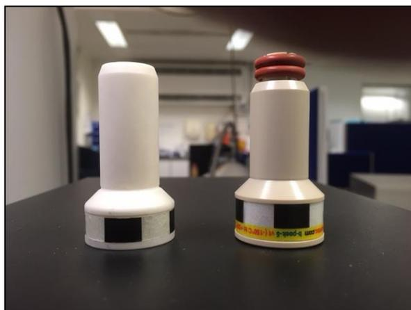
**Figure 1:** Appropriate spinners for VT NMR (*Left: ceramic, Right: PEEK*).
