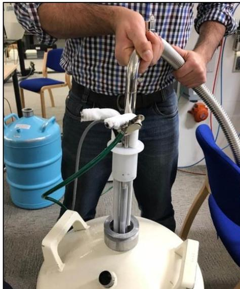
**Figure 15:** Inserting the N<sub>2</sub> exchanger into the LN<sub>2</sub> Dewar.
