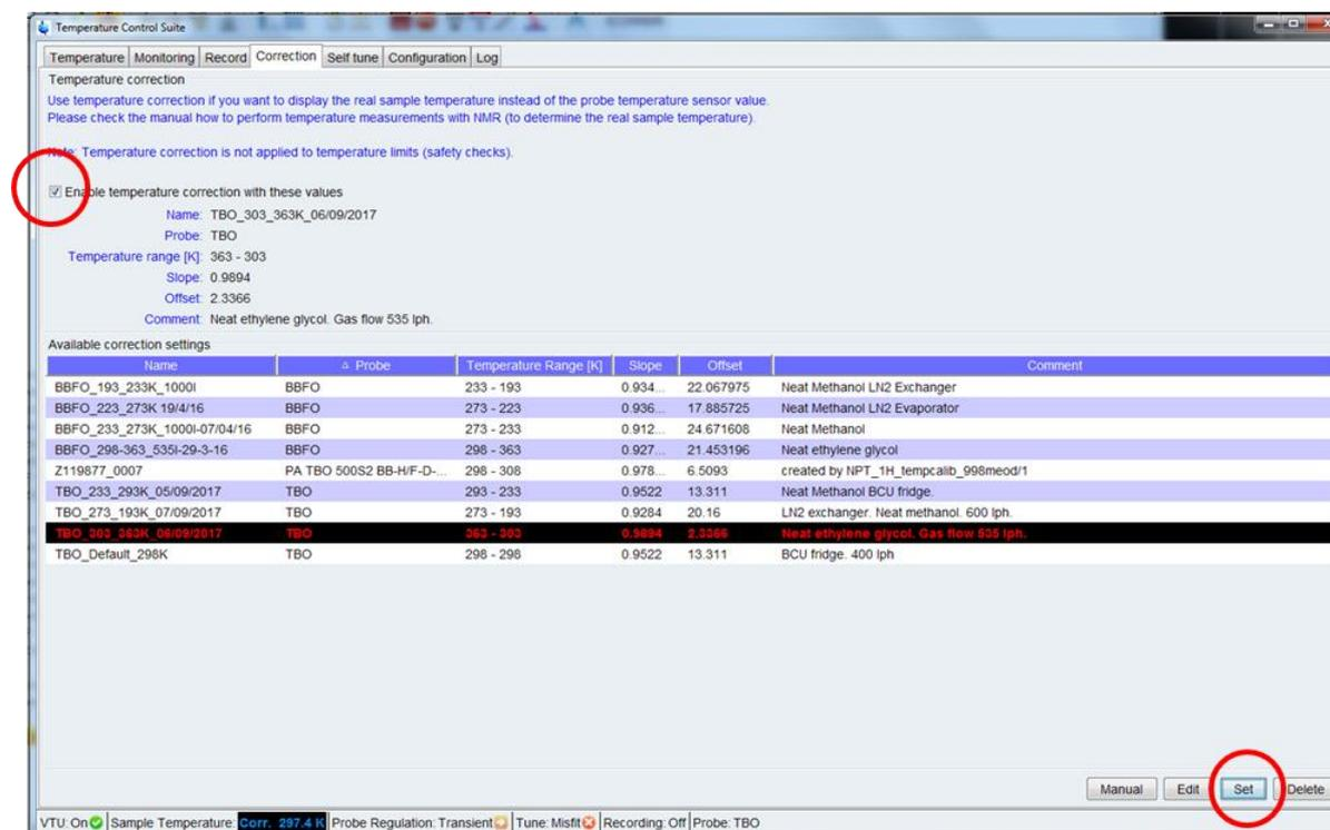
**Figure 6:** Setting the temperature calibration file.
