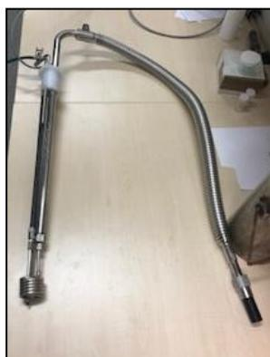
**Figure 11:** Nitrogen exchanger and transfer line for low temperature NMR.
