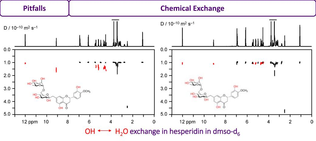
Exchange during the diffusion delay of the Oneshot45 stimulated echo leads to averaging of diffusion coefficients. Exchange in PROJECTED (PROJECT Extended for DOSY) leads only to signal loss, not to diffusion averaging, because the magnetization remains transverse during the diffusion delay.
