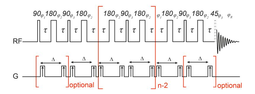
Adding gradient pulses to the PROJECT sequence to give diffusion weighting allows spin echo DOSY experiments free of J modulation. For small molecules this improves sensitivity, but also, for  $\Delta v \tau >> 1 >> k\tau$  it suppresses the averaging of diffusion coefficients for exchanging signals.
