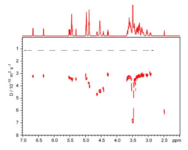
$OH/H_2O$  exchange in a convecting 30 °C solution of maltotriose in dmso-d<sub>6</sub>
