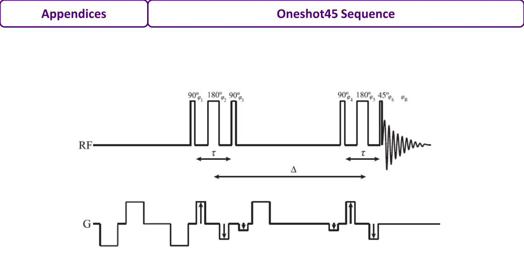
Fig. 2. Oneshot45 pulse sequence, which consists of Oneshot plus a 45° pulse orthogonal to the preceding 90° pulse.
