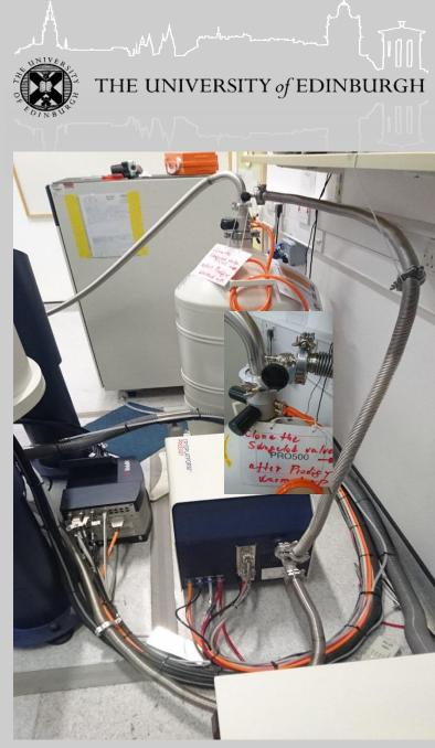
After - continuous (Swagelog valve opened) pumping of TFL using CryoPlatform turbo pump
